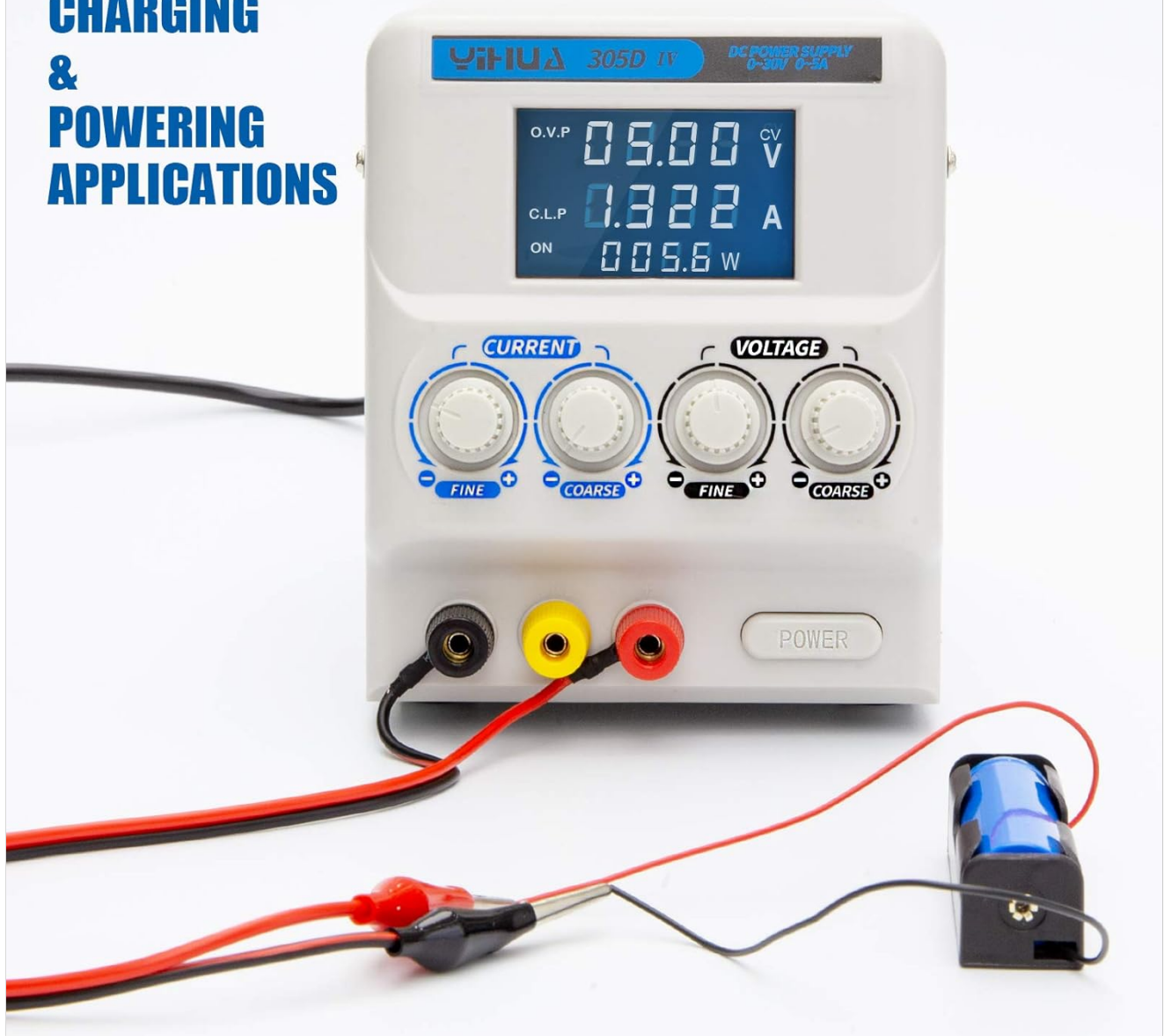
Image 5.4: YIHUA 305D-IV used for charging or powering applications.
