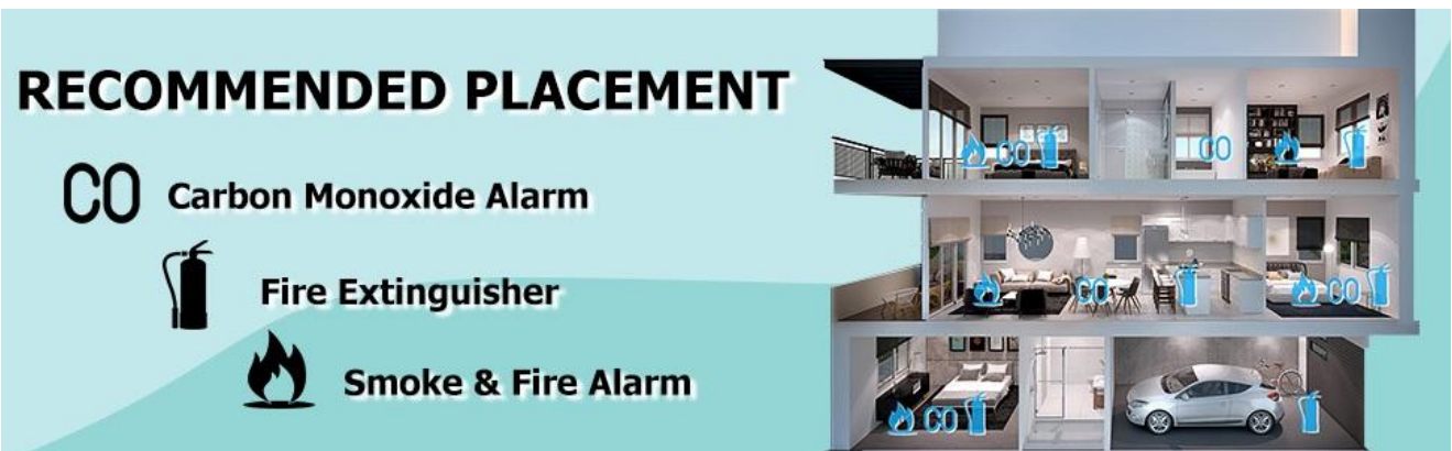
Image 9: A cross-section diagram of a multi-story house indicating optimal locations for Carbon Monoxide Alarms (CO) on each floor and near bedrooms.
