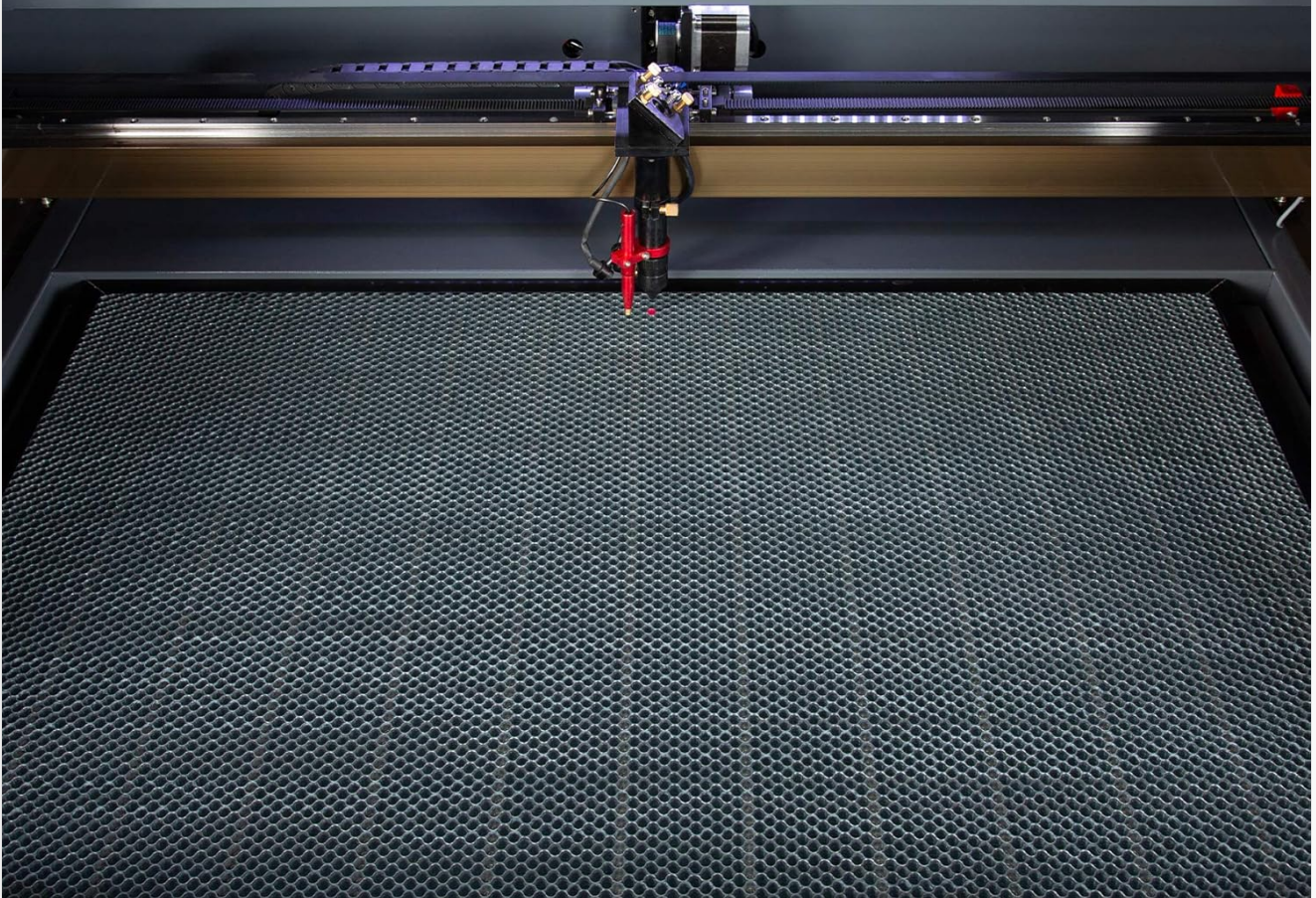
Figure 9.1: The spacious 16" x 30" engraving area, providing over 3.3 square feet for projects.
