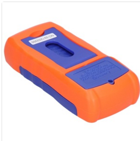
Image 4.1: Back view of the meter, indicating the battery compartment.
