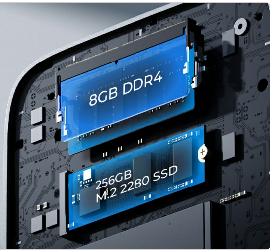
Image 5.3: The Mini PC's internal layout, showing the integrated RAM and M.2 SSD, with space for a 2.5-inch drive.
