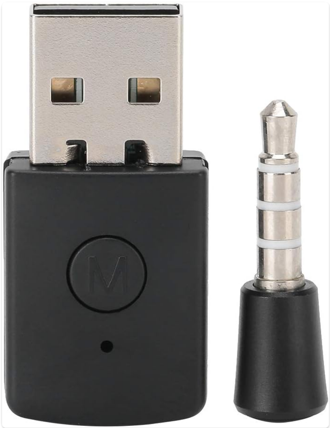
Image 1.1: The ASHATA Bluetooth Adapter (USB dongle) and its accompanying 3.5mm microphone jack. The dongle features a button and an indicator light.
