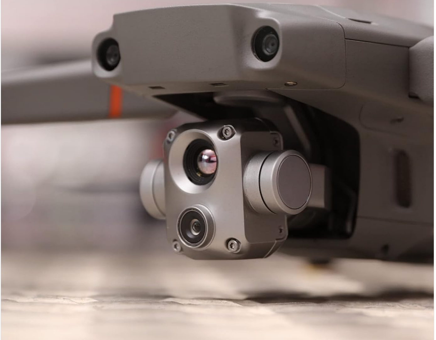
Image: A detailed view of the drone's gimbal, showcasing the integrated visual and thermal cameras.
