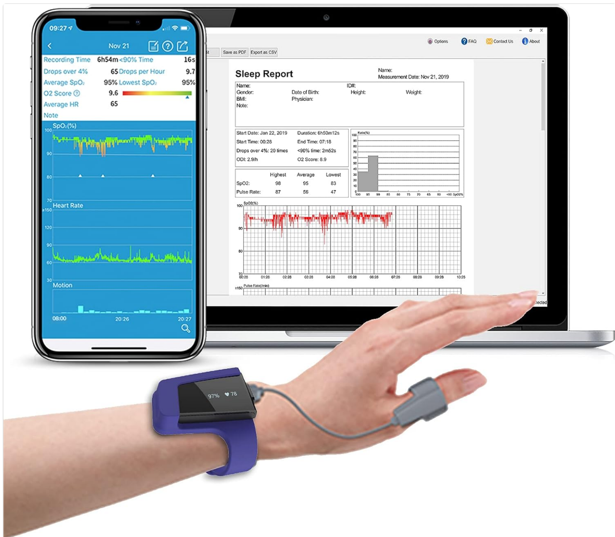
Figure 5: The Wellue wrist monitor and sensor ring in operation, showing real-time data on a smartphone and a comprehensive sleep report generated on a laptop.
