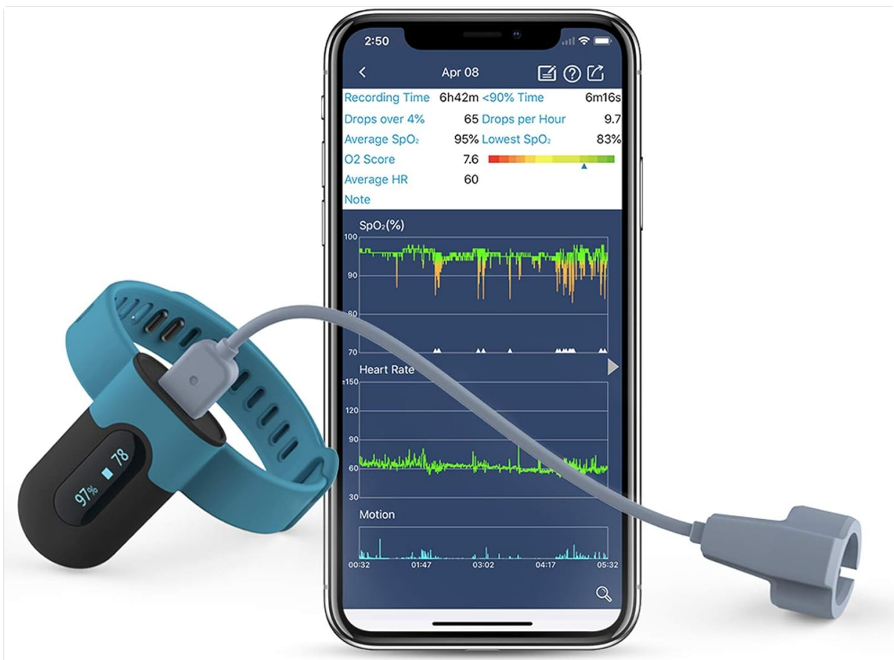
Figure 4: An illustration of the Wellue wrist monitor, to which the sensor ring connects, displaying sleep data on a smartphone application.
