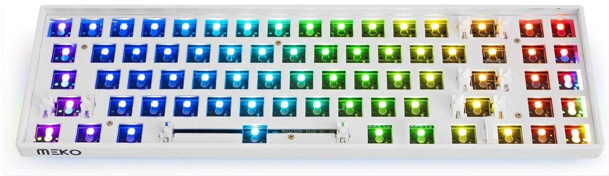
Image: Internal view of the MEKO Push keyboard, showing the hotswap sockets ready for switch installation.
