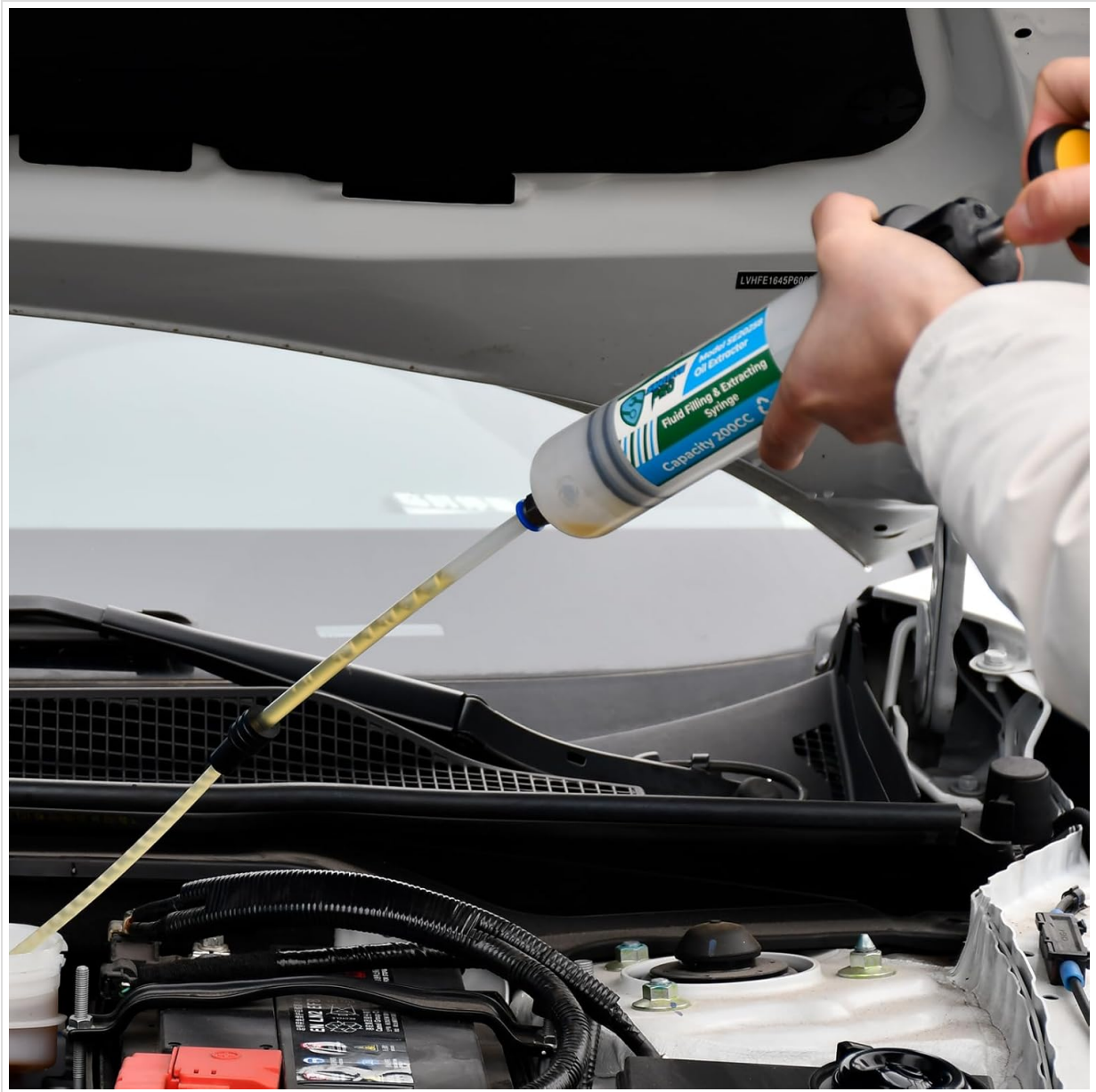
Figure 5: The SMOTIVEPRO pump in action, demonstrating fluid extraction from a vehicle's reservoir within the engine bay, highlighting its ease of use in confined spaces.
