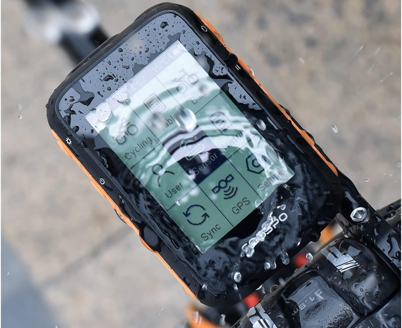
Image 8.1: The BC200 demonstrating its IP67 waterproof capability under water spray.
