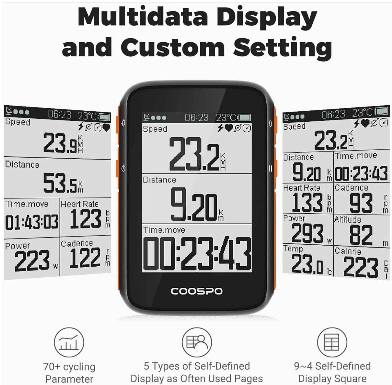
Image 5.1: Various customizable data display layouts on the BC200 screen, showing speed, distance, time, heart rate, power, cadence, altitude, temperature, and calories.
