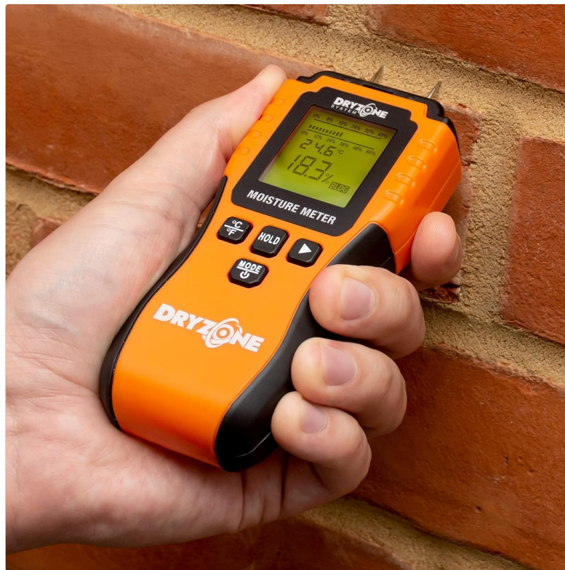
Figure 4.1: Measuring moisture in building materials.
