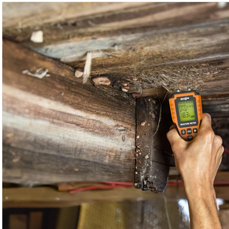
Figure 4.2: Measuring moisture in wood.
