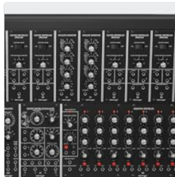
Figure 2.4: Close-up detail of various modules within the SYSTEM 55, including Voltage Controlled Oscillators and Envelope Generators.
