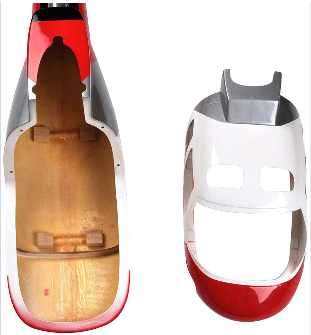
Image: The AS350 Ecureuil fuselage separated into its two main halves, illustrating the internal structure and mounting points for the helicopter chassis.
