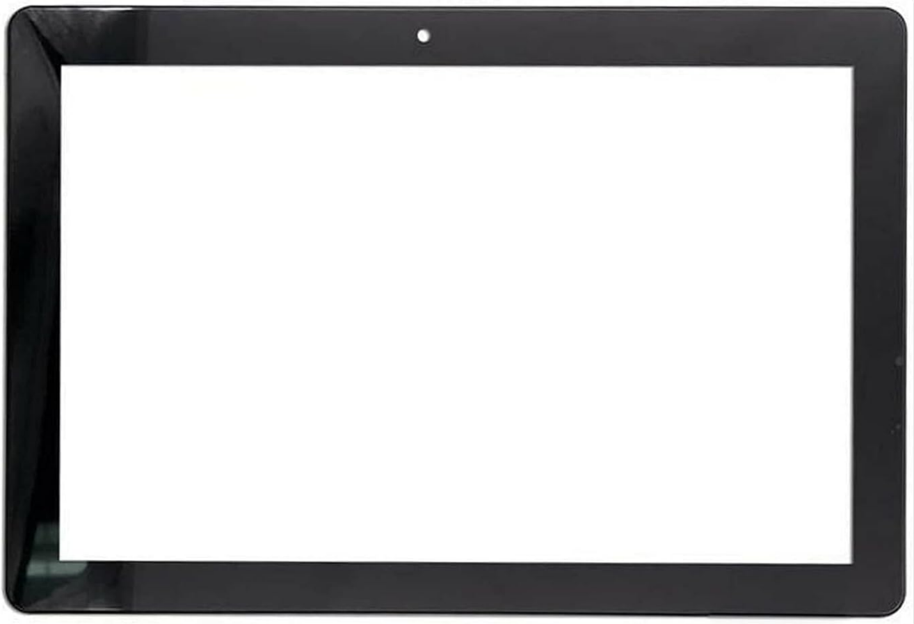
Image 2.1: A clear front view of the 10.1-inch touch screen digitizer panel, showing its rectangular shape and the cutout for the front camera. This is the primary component for touch input.
