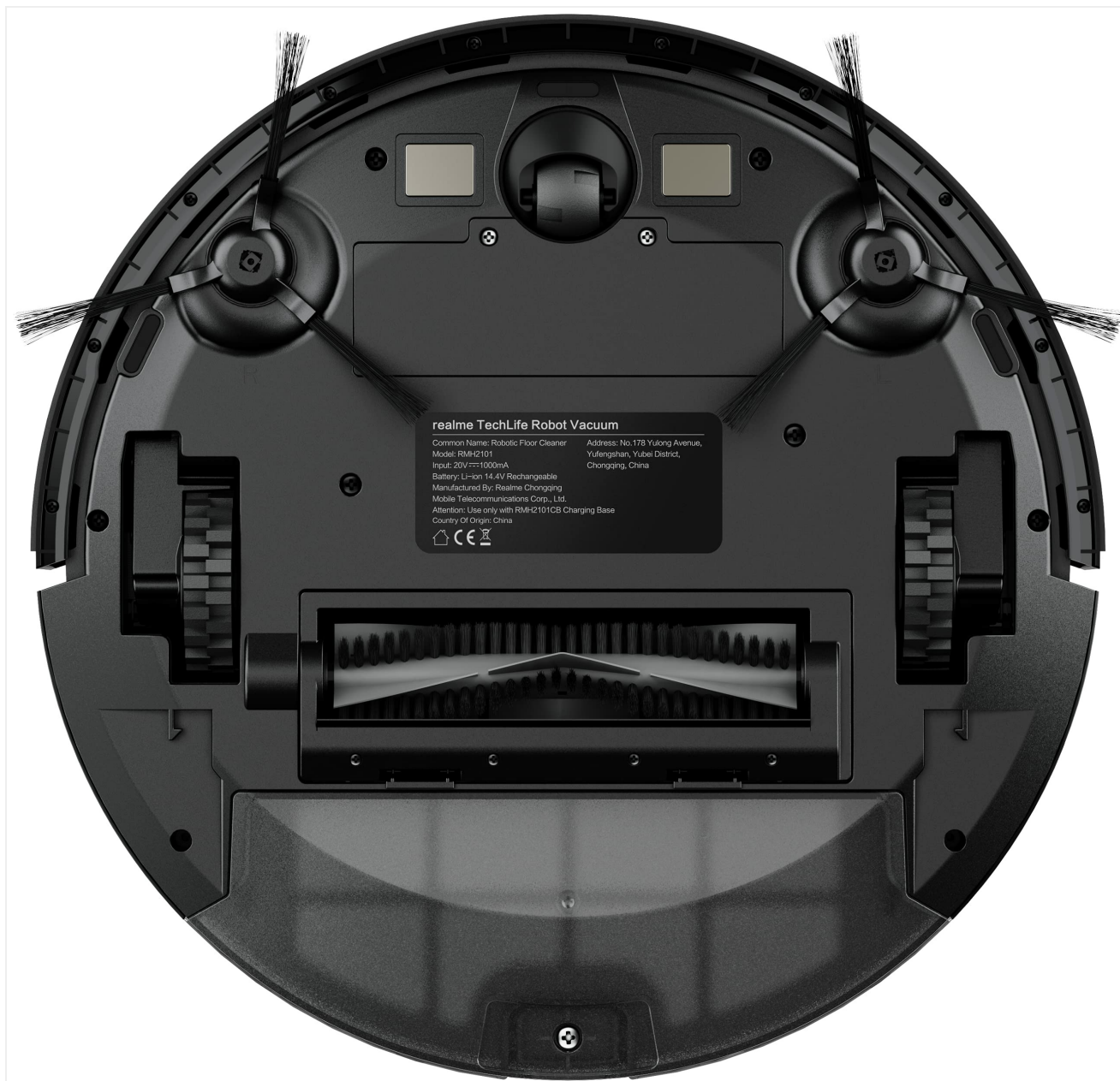
The underside of the robot vacuum, displaying the main brush, side brushes, and wheels.
