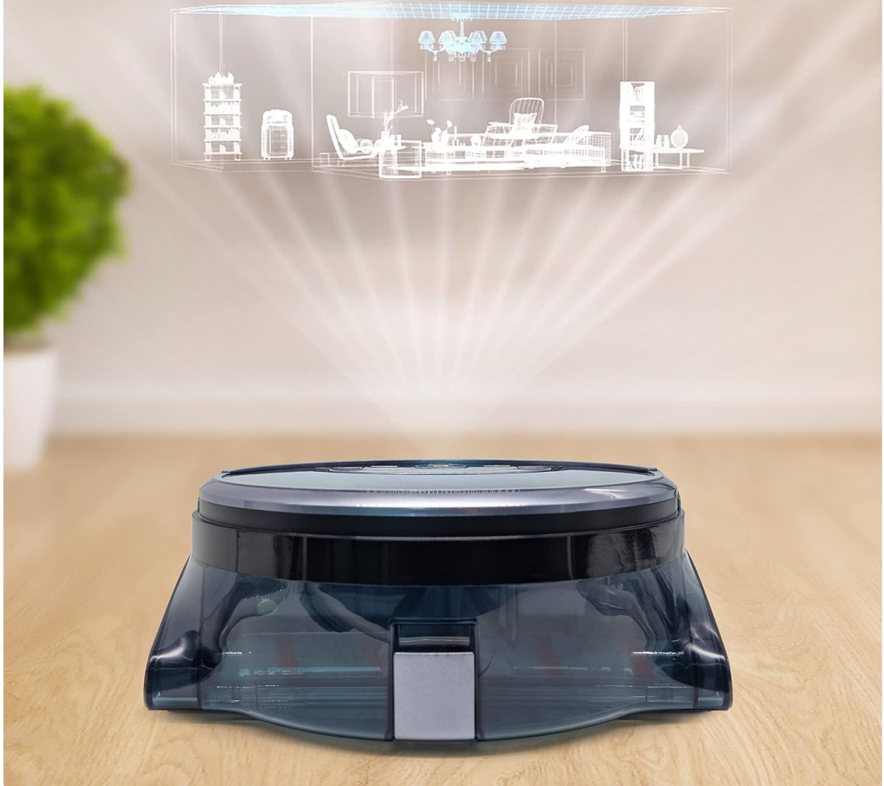
Figure 3.3: Depiction of the robot's 360-degree camera navigation system, which maps the cleaning area for systematic coverage.
