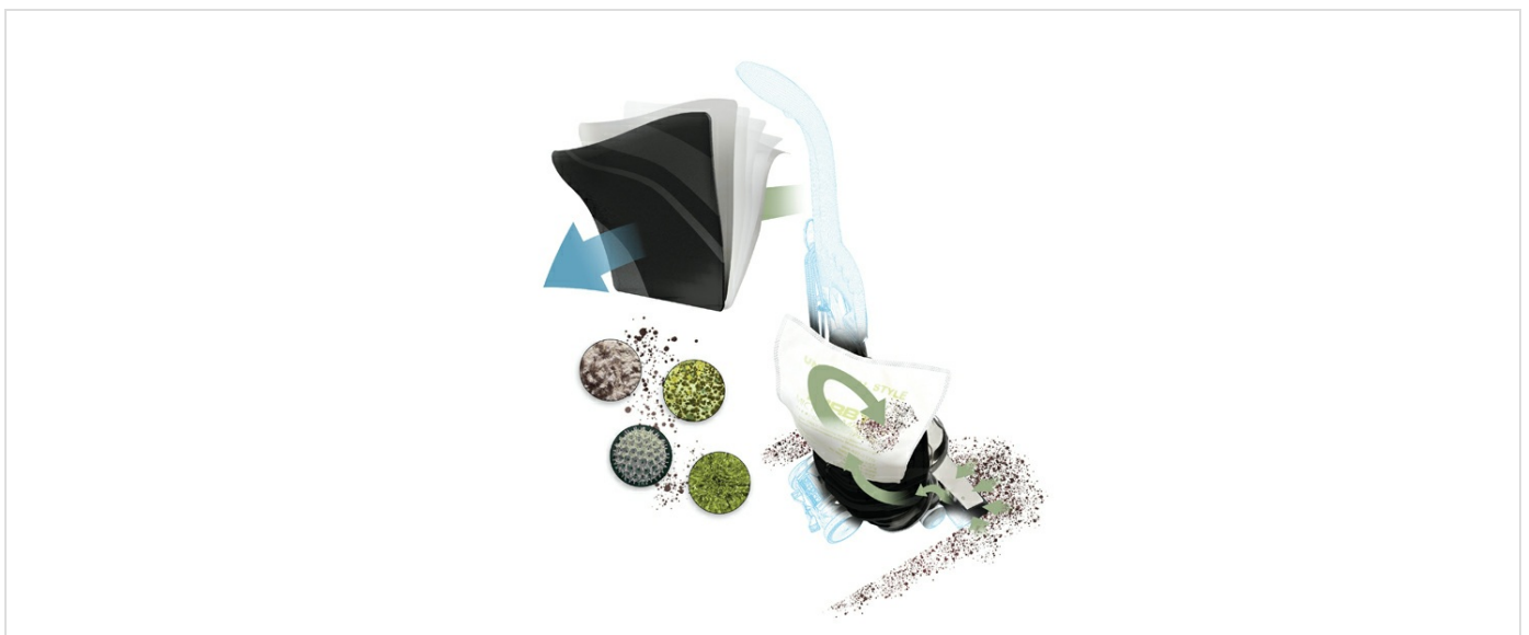
Figure 5.2: Filtration diagram detailing how dust and allergens are captured.
