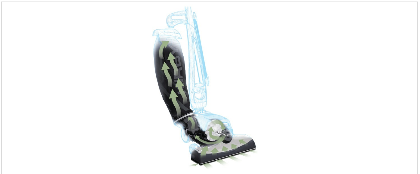
Figure 5.1: Airflow diagram showing the path of air and debris through the vacuum.
