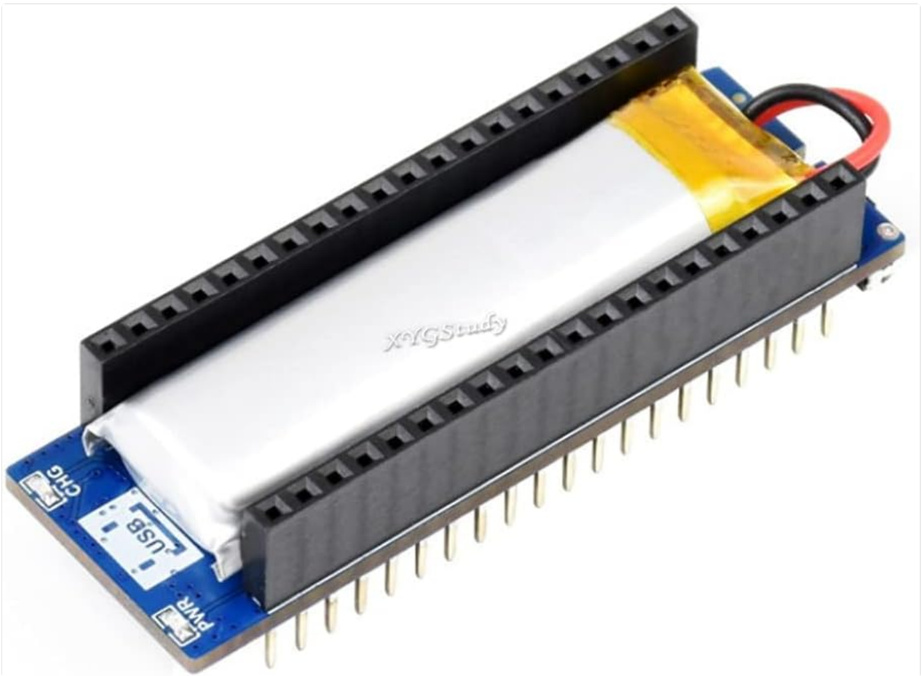
Figure 4: Pico-UPS-B module with connected Li-po battery.
