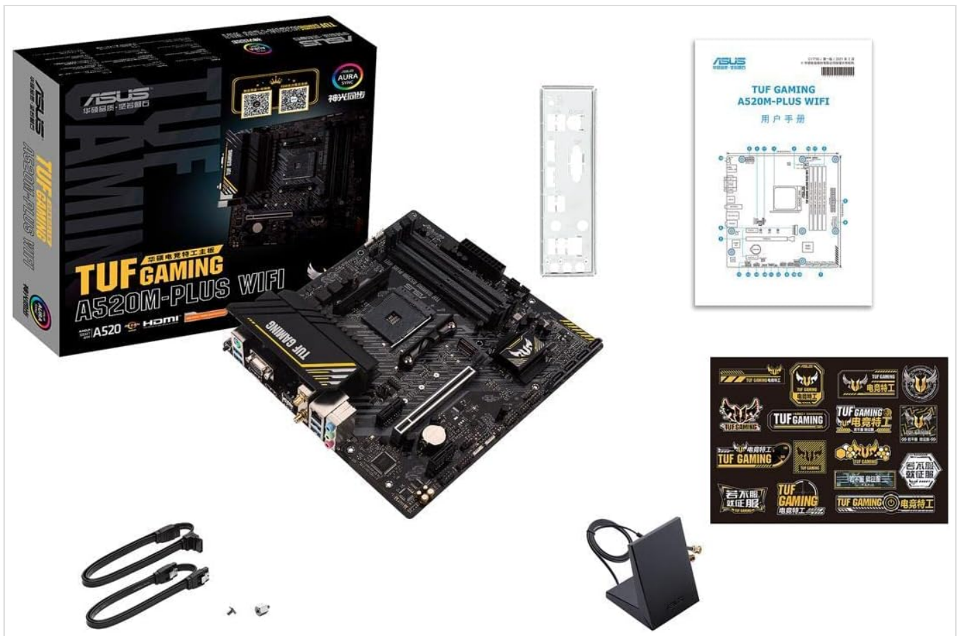
Figure 2: The motherboard packaging and its contents, including the manual, I/O shield, cables, and antenna.
