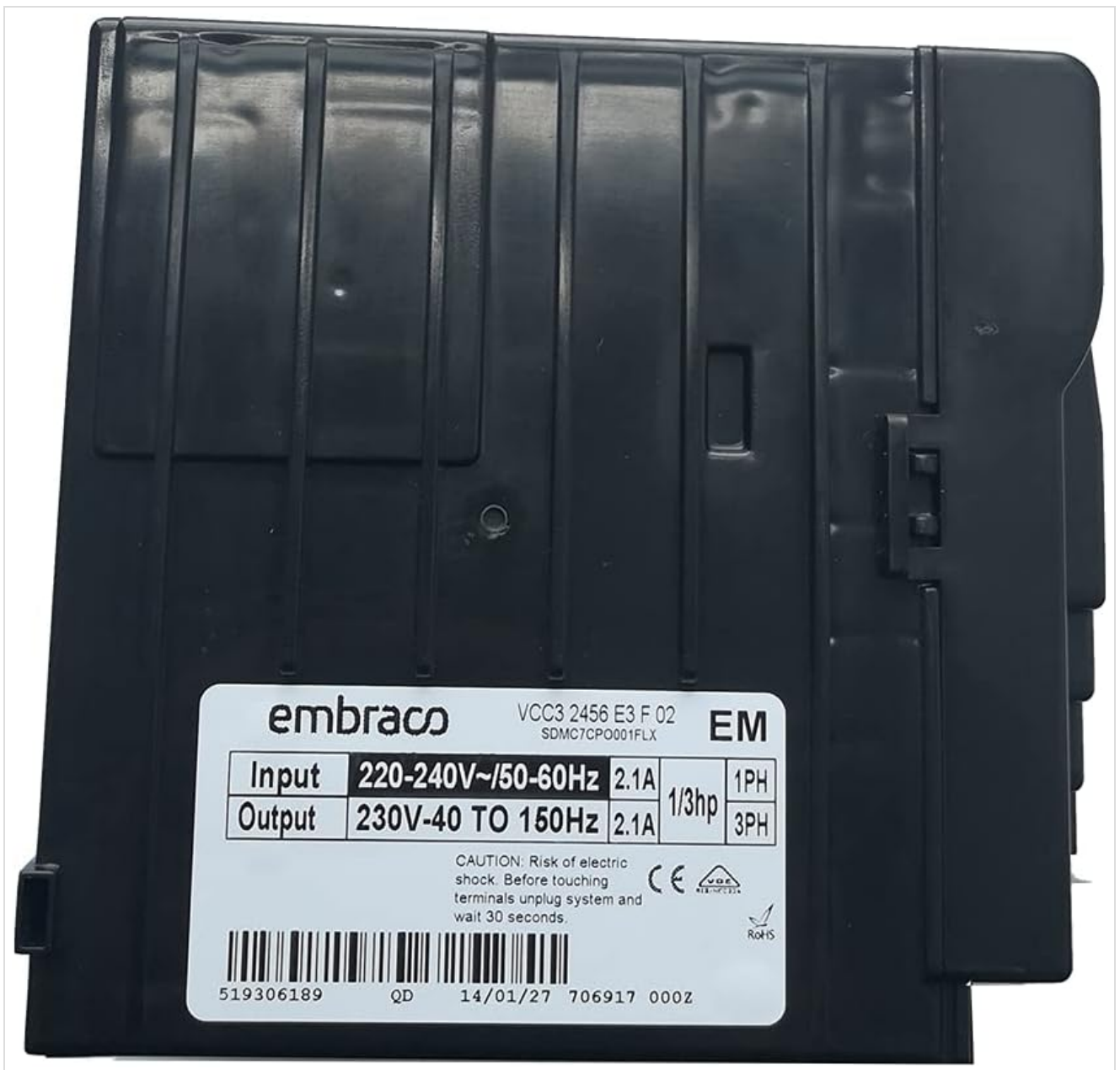
Figure 4.3: Front view of the inverter, displaying the product label with input/output specifications and safety warnings. Note the part numbers and manufacturing codes on the label.
