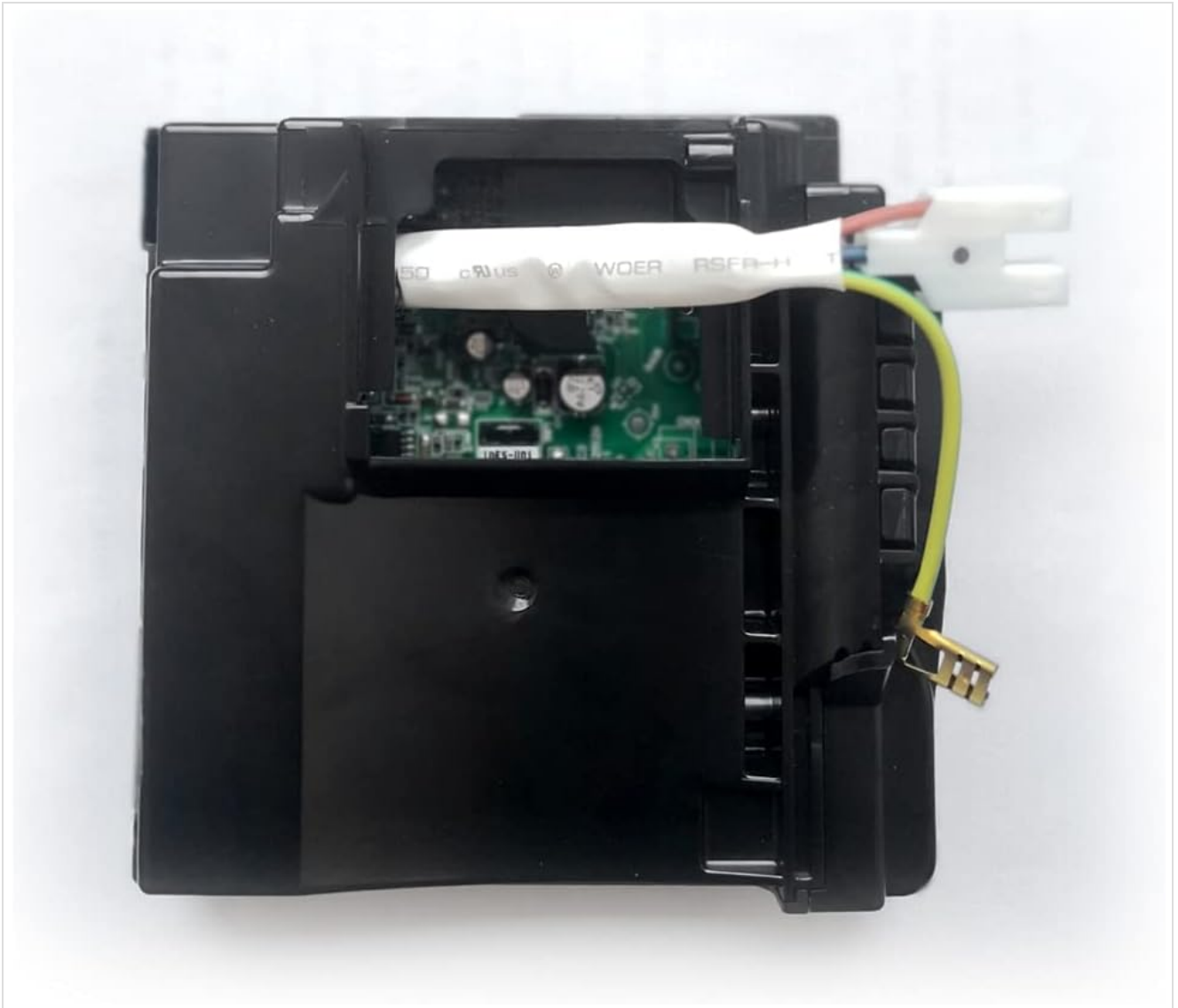
Figure 4.1: Side view of the inverter, highlighting the internal circuitry and the pre-attached wiring harness.
