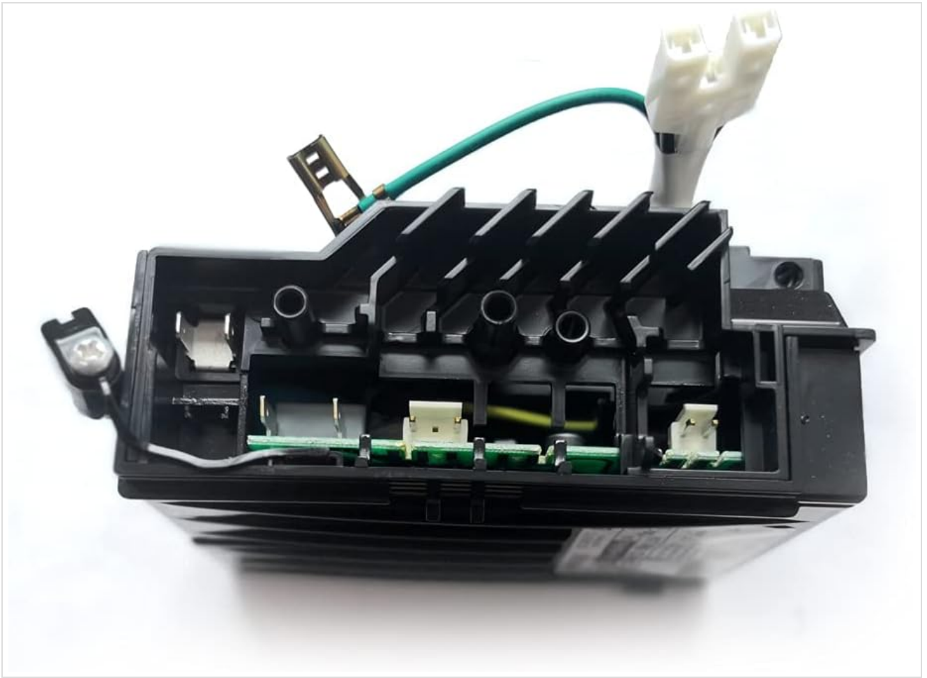
Figure 4.2: Top view of the inverter, showing the various connection points for power input and output.
