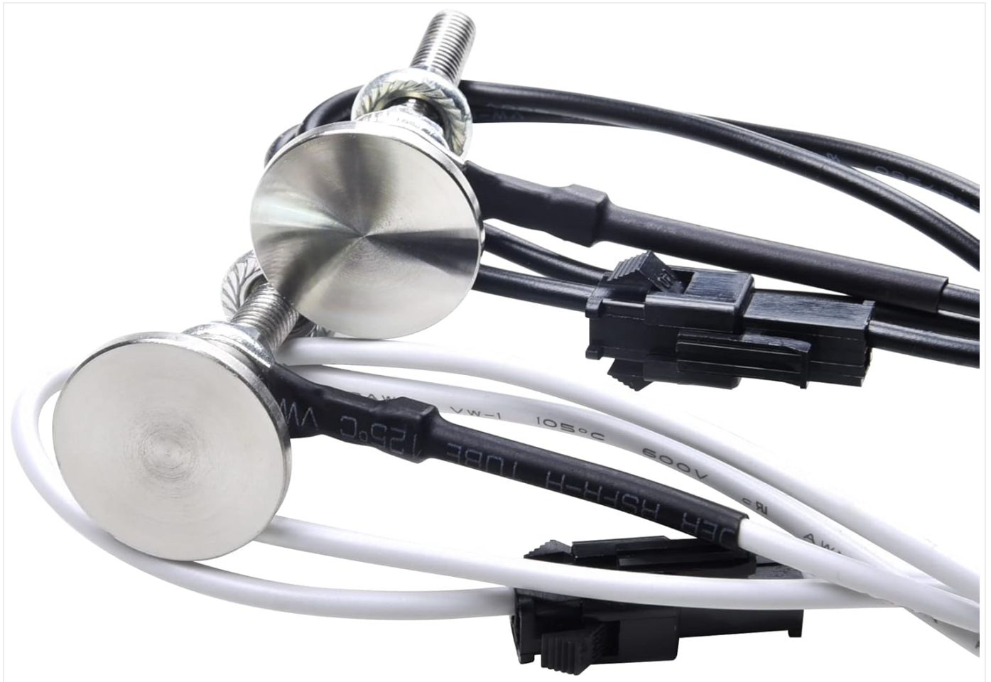
Figure 2: Detail of the two touch sensors and their associated black and white lead wires.
