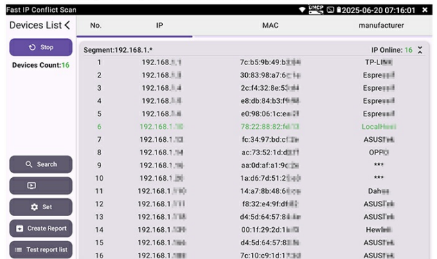
Image: Screenshots demonstrating IP Discovery (auto-scanning network segment IP addresses) and Fast IP Conflict Scan (quickly finding IP addresses and supporting MAC address, camera manufacturer, and IP conflict resolution).
