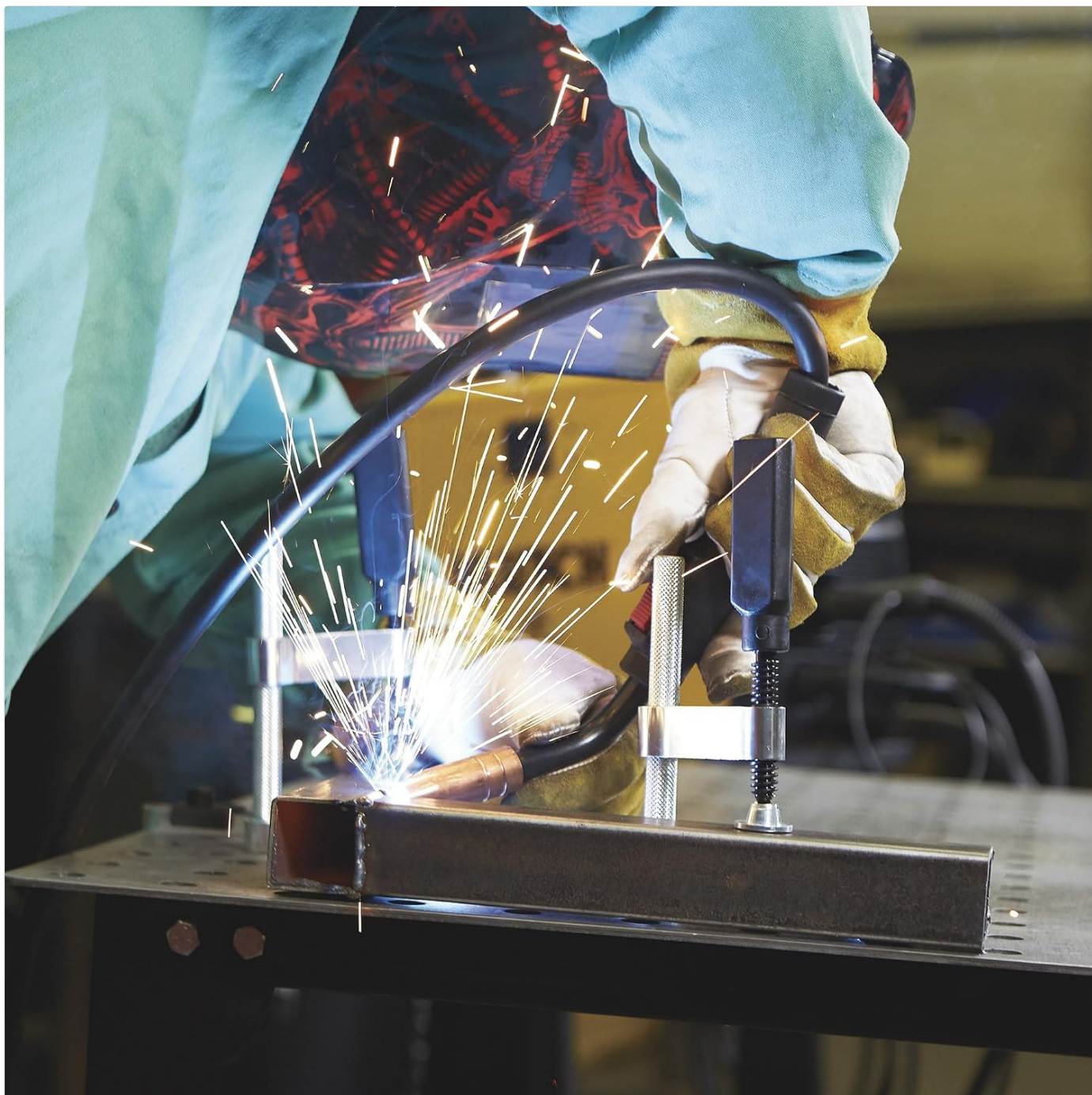
Image: A close-up of a corner joint being welded, illustrating how multiple clamps can be used simultaneously for complex setups.
