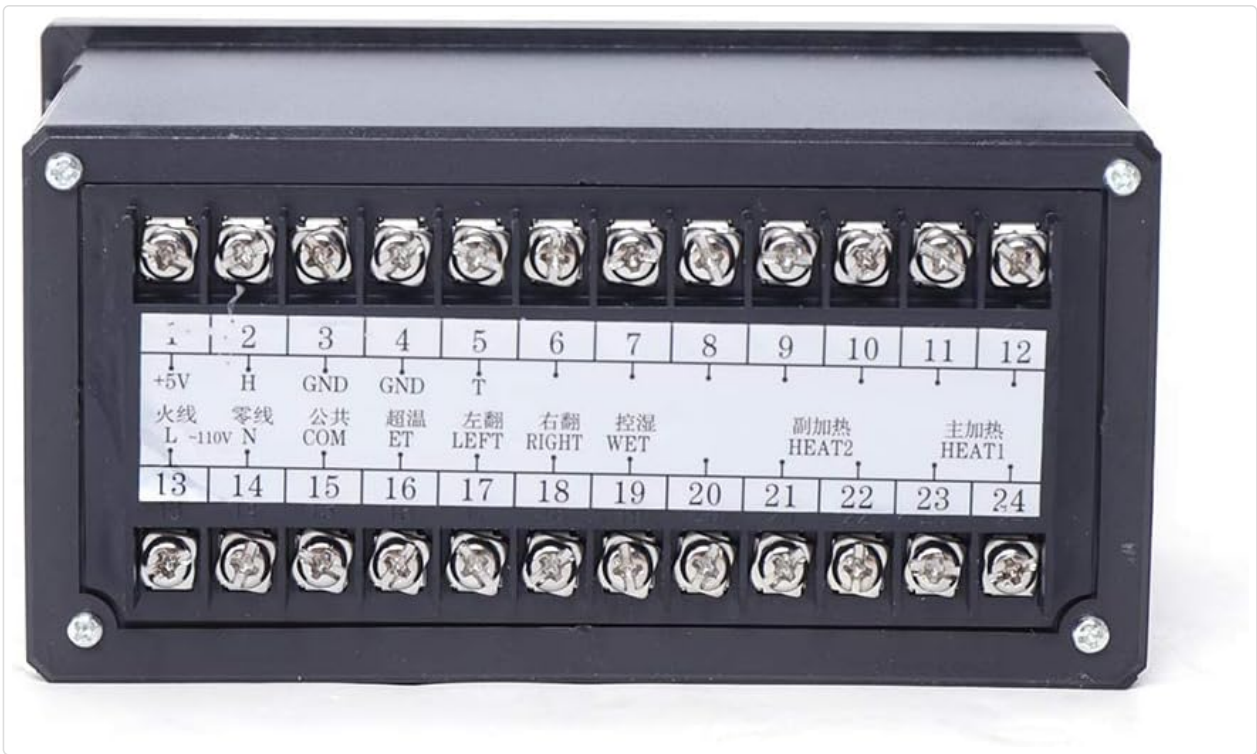
Image: Rear view of the XM-18 Controller with wiring terminals.
