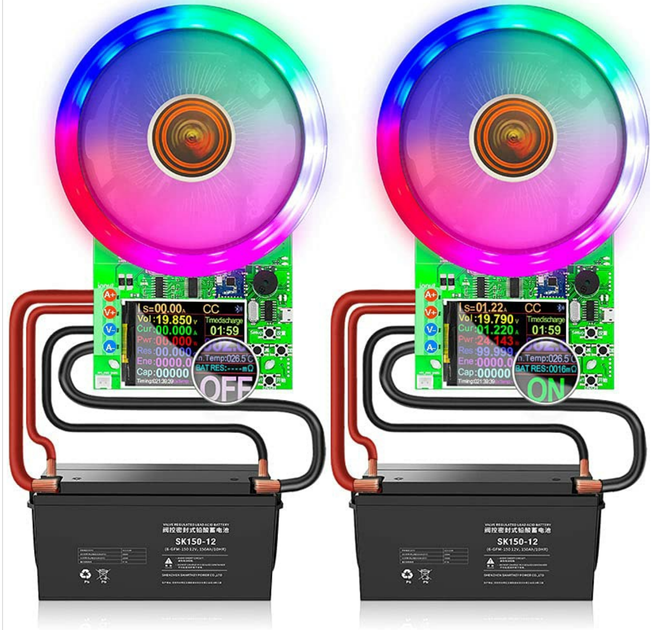
Figure 5.2: Setting timed constant current discharge and cut-off voltage.
