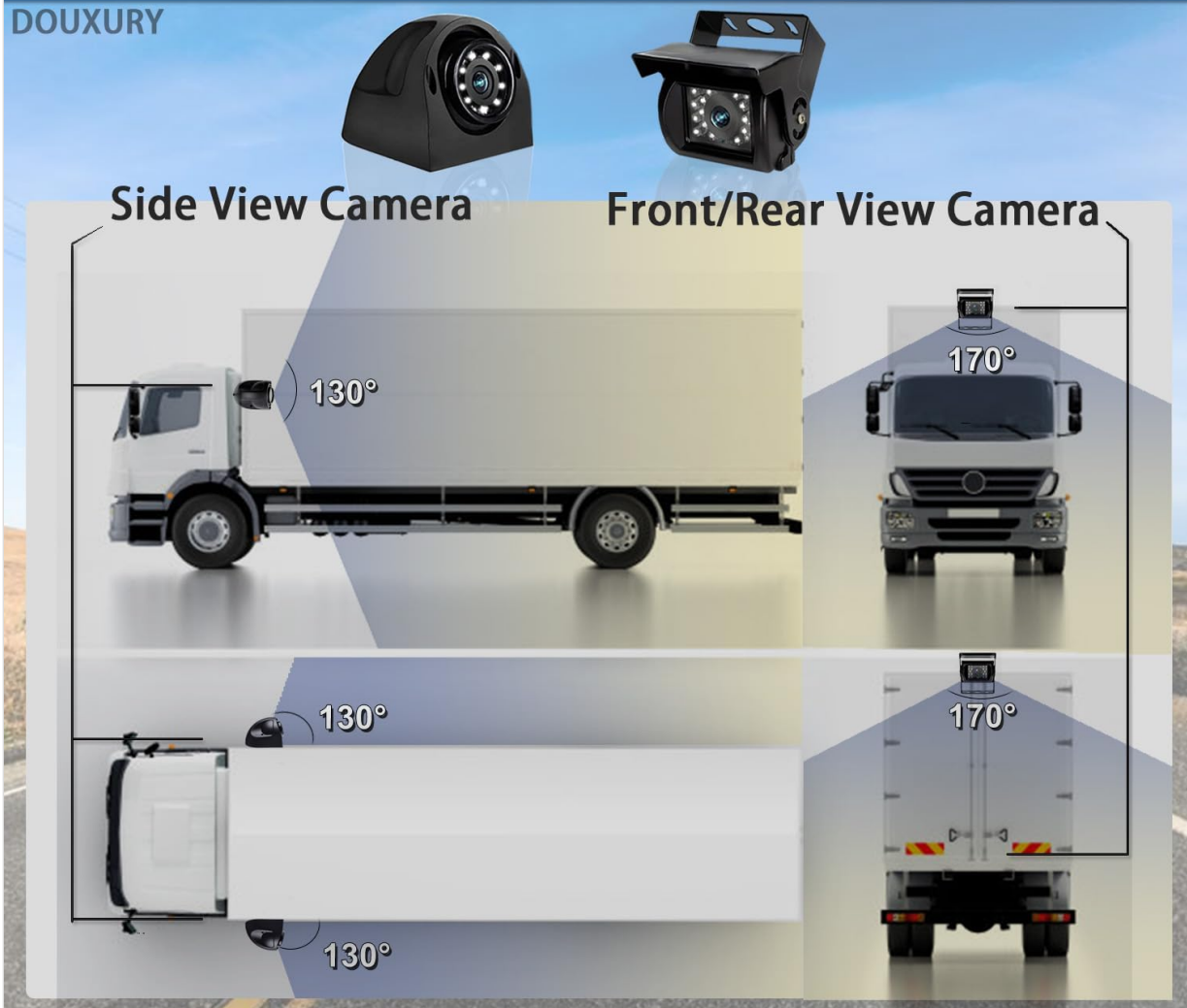
Figure 3.3: Recommended camera placement for front/rear (170° view) and side (130° view) cameras to achieve comprehensive coverage.
