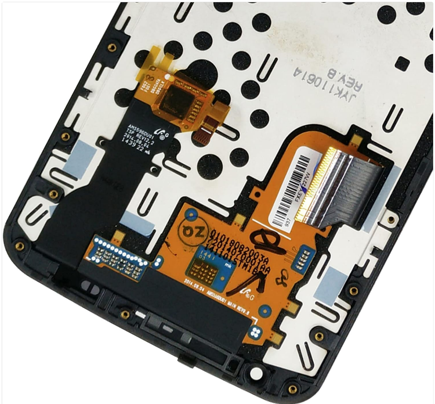
Image 4.3: Detailed view of the flex cables and connectors, crucial for proper installation.
