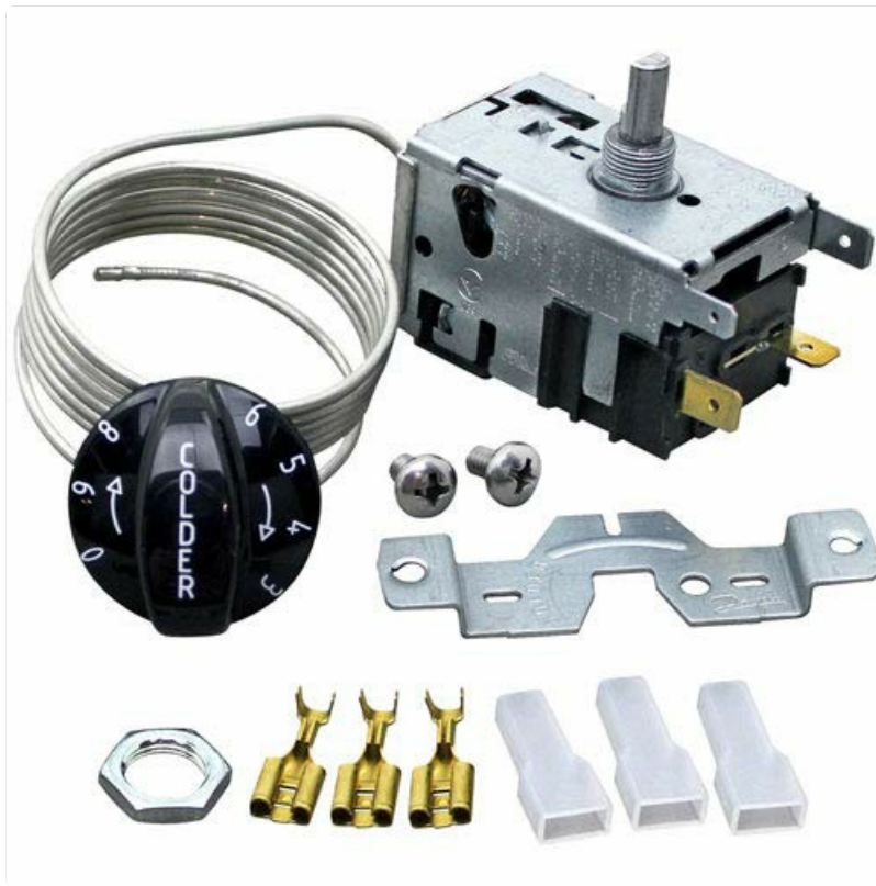
Figure 1: Complete Mavrik 077B7061 Temperature Control Kit. This image displays the main control unit with its D-stem shaft, a coiled 36-inch capillary tube, a black temperature adjustment dial marked 'Colder' with settings 1-9, a metal mounting bracket, two screws, and three 1/4-inch T-connectors with white insulators.
