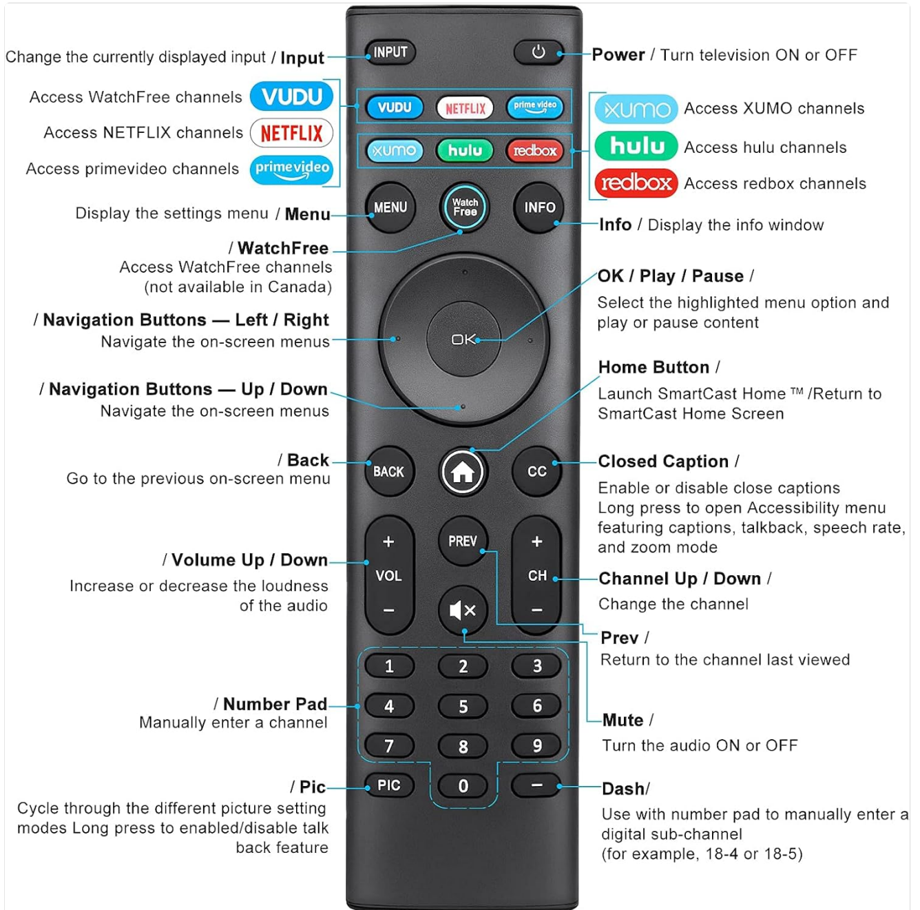
Image: Detailed diagram of the EWO'S XRT140 remote control, labeling each button with its corresponding function.
