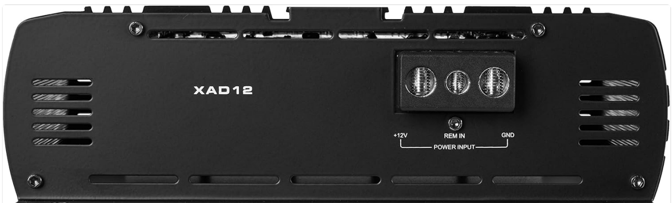
Figure 3.2: Rear view of the NVX XAD12 amplifier, detailing the power input section with +12V, REM IN, and GND terminals clearly labeled.
