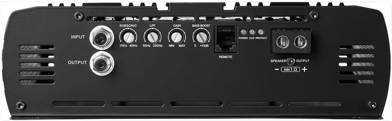
Figure 4.2: Top view of the NVX XAD12 amplifier, providing a clear look at the Subsonic, LPF, Gain, and Bass Boost controls, along with the POWER/CLIP/PROTECT indicators.
