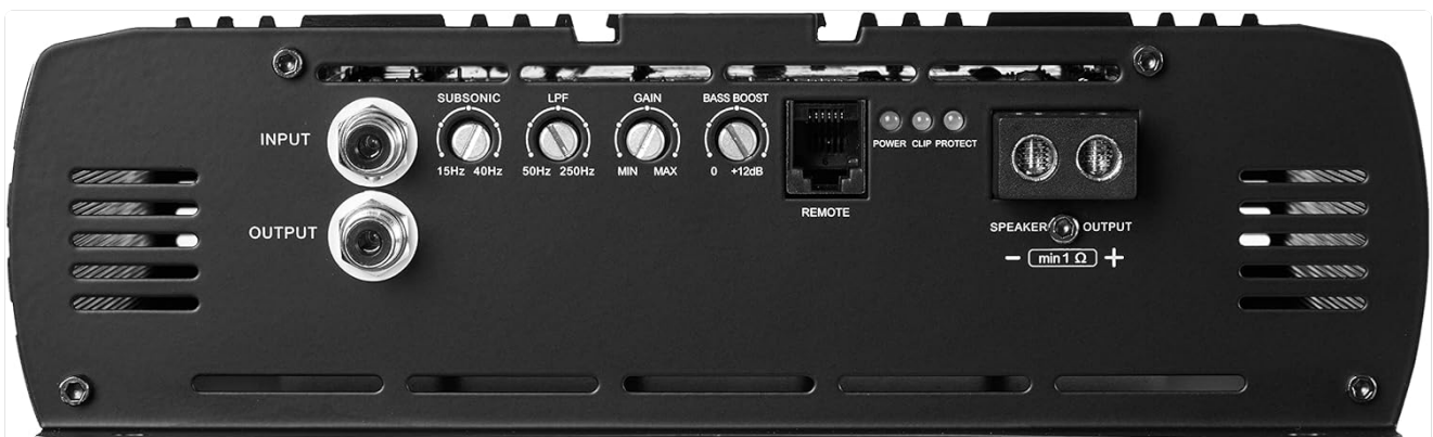
Figure 3.4: Top view of the NVX XAD12 amplifier, illustrating the RCA input and output connections, along with various control knobs for audio adjustment.
