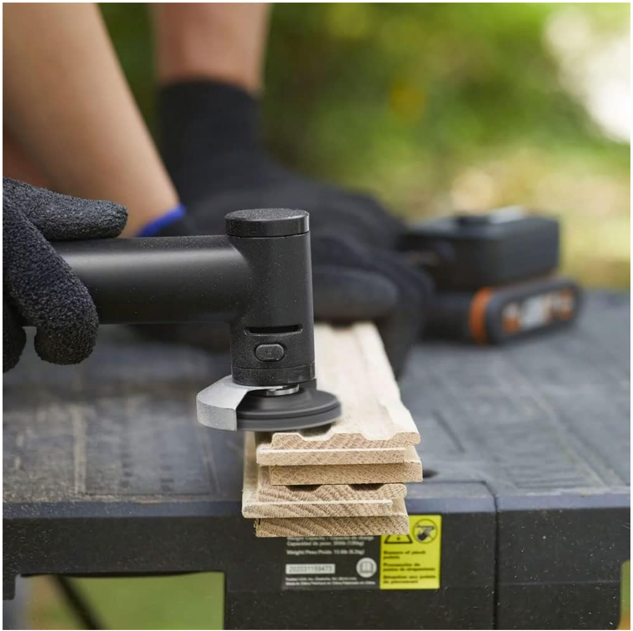
Image 5.5: The MakerX Mini Grinder equipped with a sanding attachment, being used to smooth a wooden surface.
