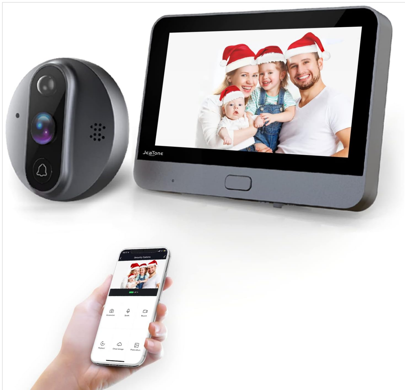
Image: Overview of the JeaTone Peephole Viewer system, showing the outdoor camera, indoor monitor, and smartphone app.
