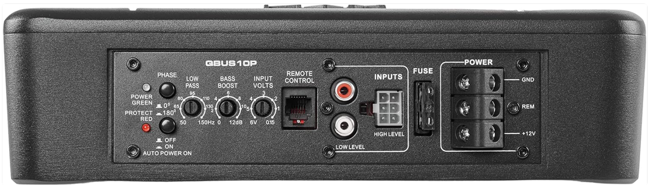
Figure 2.2: Rear panel of the NVX QBUS10P, showing power, input, and control connections.
