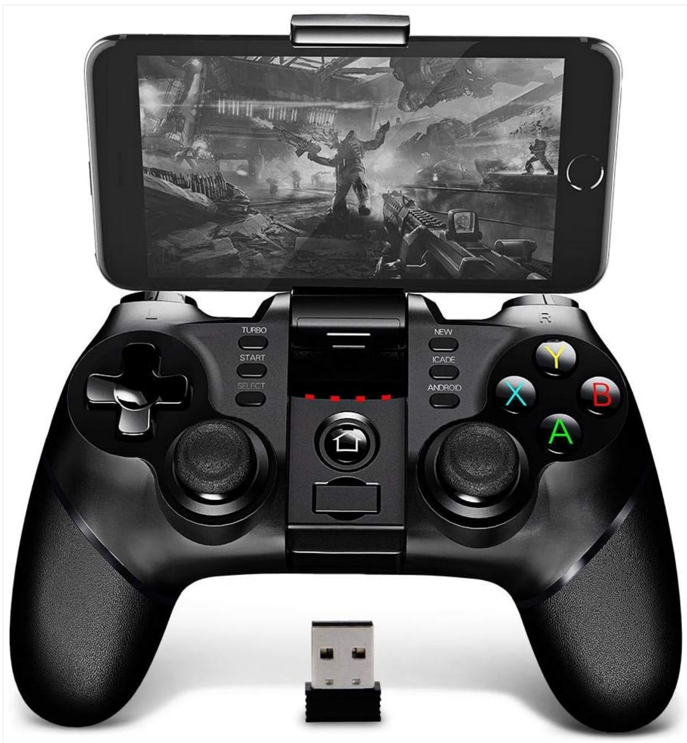
Figure 4.2: The iPega PG-9076 Gamepad with a smartphone attached, and the 2.4G USB wireless receiver prominently displayed in the foreground. This illustrates the wireless connectivity option for devices like PCs and TV boxes.
