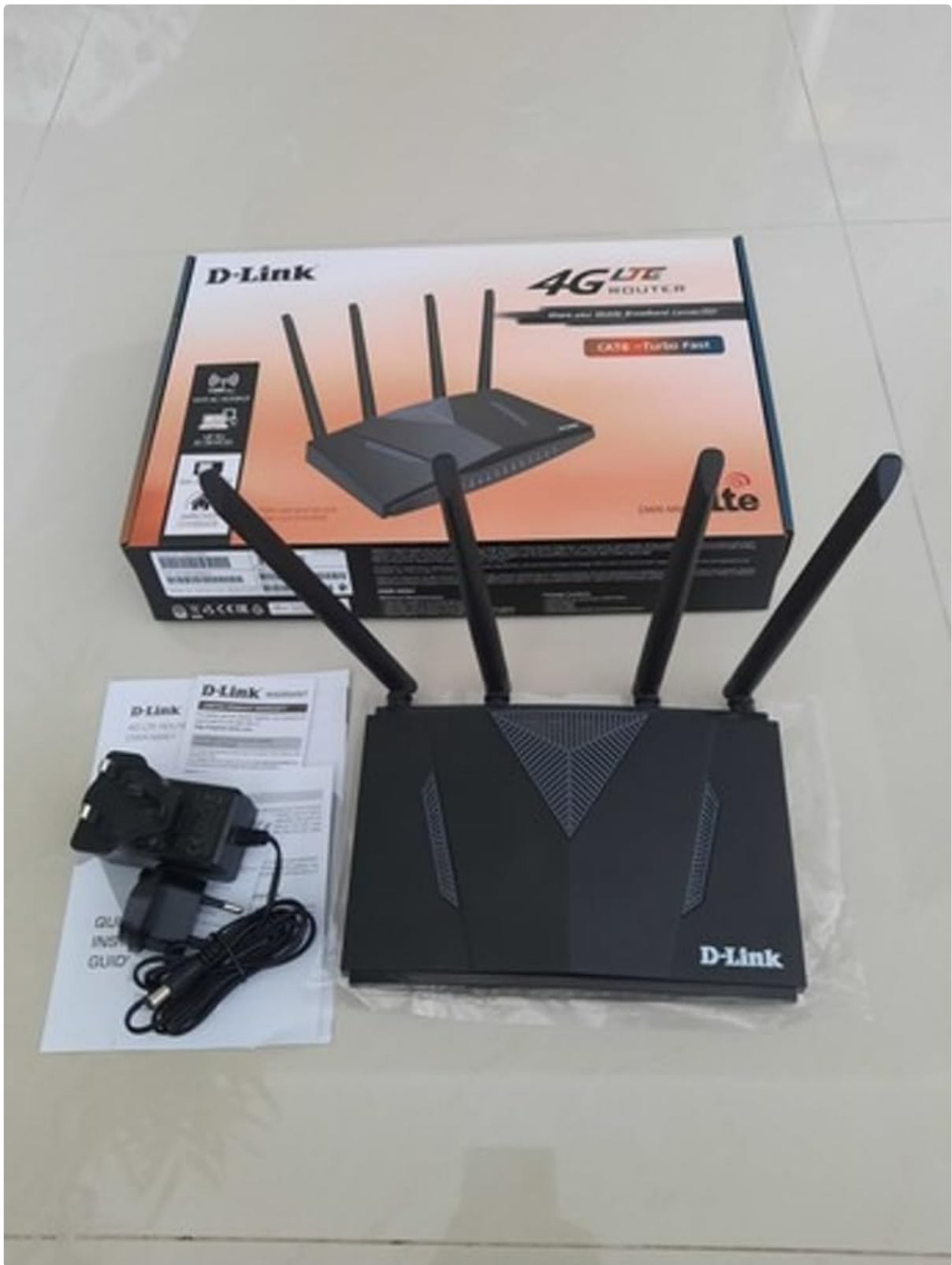
Figure 2.1: Package Contents. This image shows the DWR-M960 router, its power adapter, and the quick installation guide, all laid out next to the product box.
