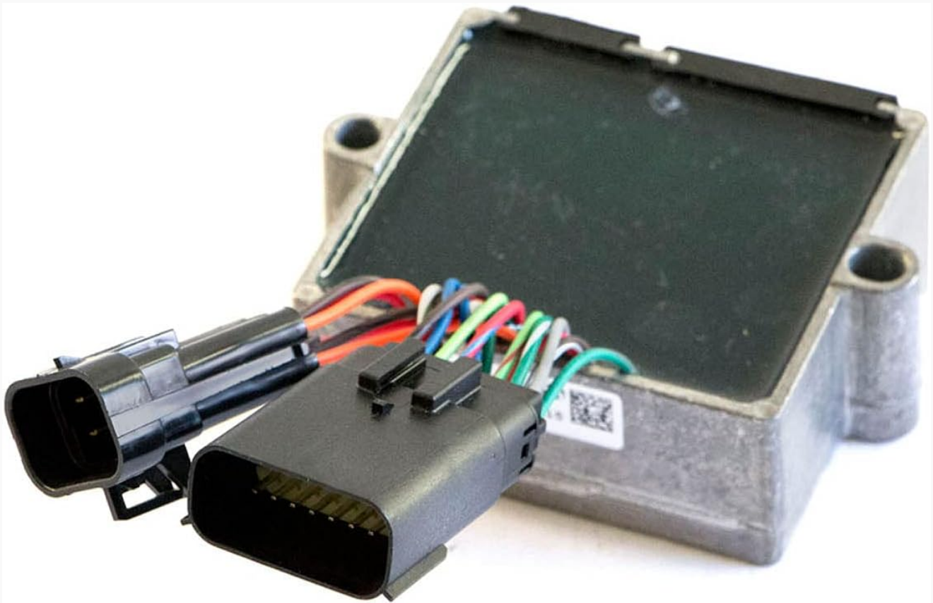
Angled view of the VCM, highlighting the connector ports and module casing.
