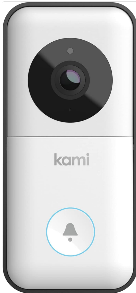
Figure 1: Front view of the Kami Smart Video Doorbell Camera, showing the camera lens, Kami logo, and doorbell button.
