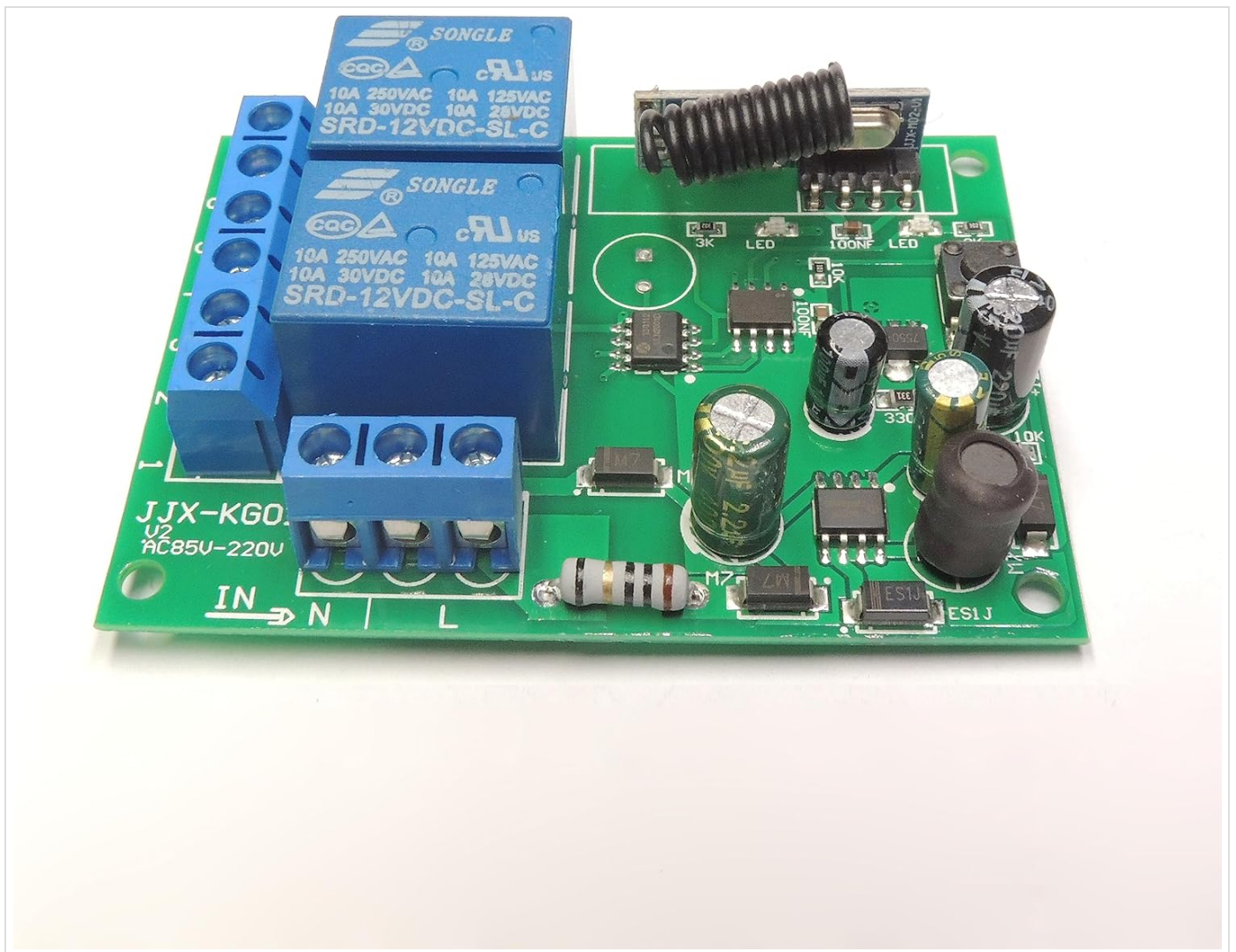
Image: A close-up view of the DieseRC receiver board, highlighting the learning button used for pairing remote controls.
