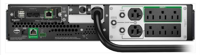
The rear panel provides the input power connection (NEMA 5-20P), eight NEMA 5-15R output receptacles, and two NEMA 5-20R output receptacles. Communication ports include USB, serial, and an Ethernet port for the integrated Network Management Card. An Emergency Power Off (EPO) port is also available for remote shutdown.
