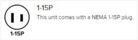
Figure 3: Diagram illustrating the NEMA 1-15P plug type, indicating compatibility with standard 120V outlets.
