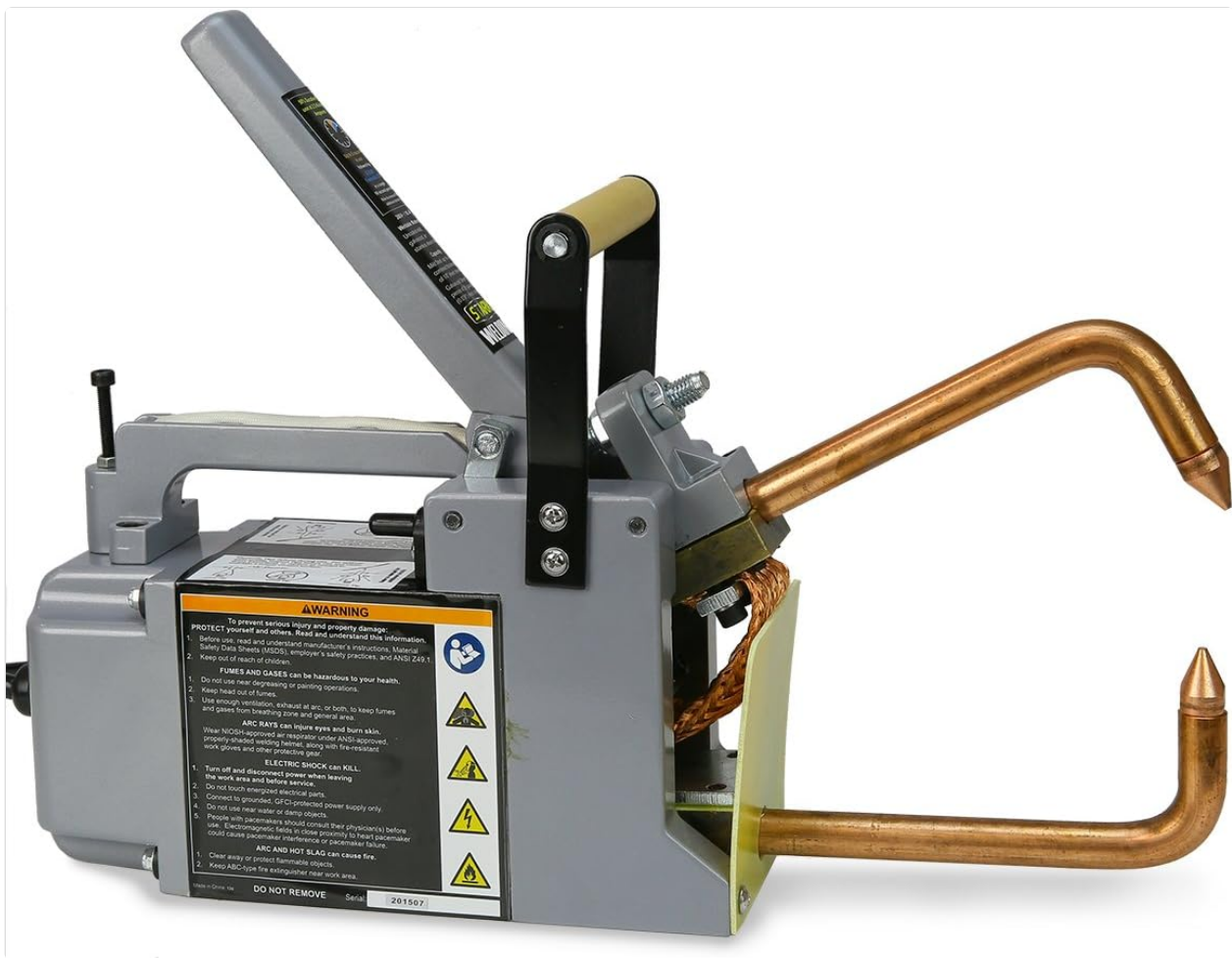
Figure 4: Side view of the spot welder with the lever in an open position, ready for material placement.
