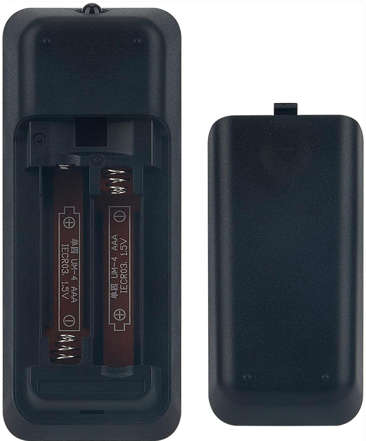
Figure 2.1: Battery compartment with two AAA batteries installed. Ensure correct polarity.
