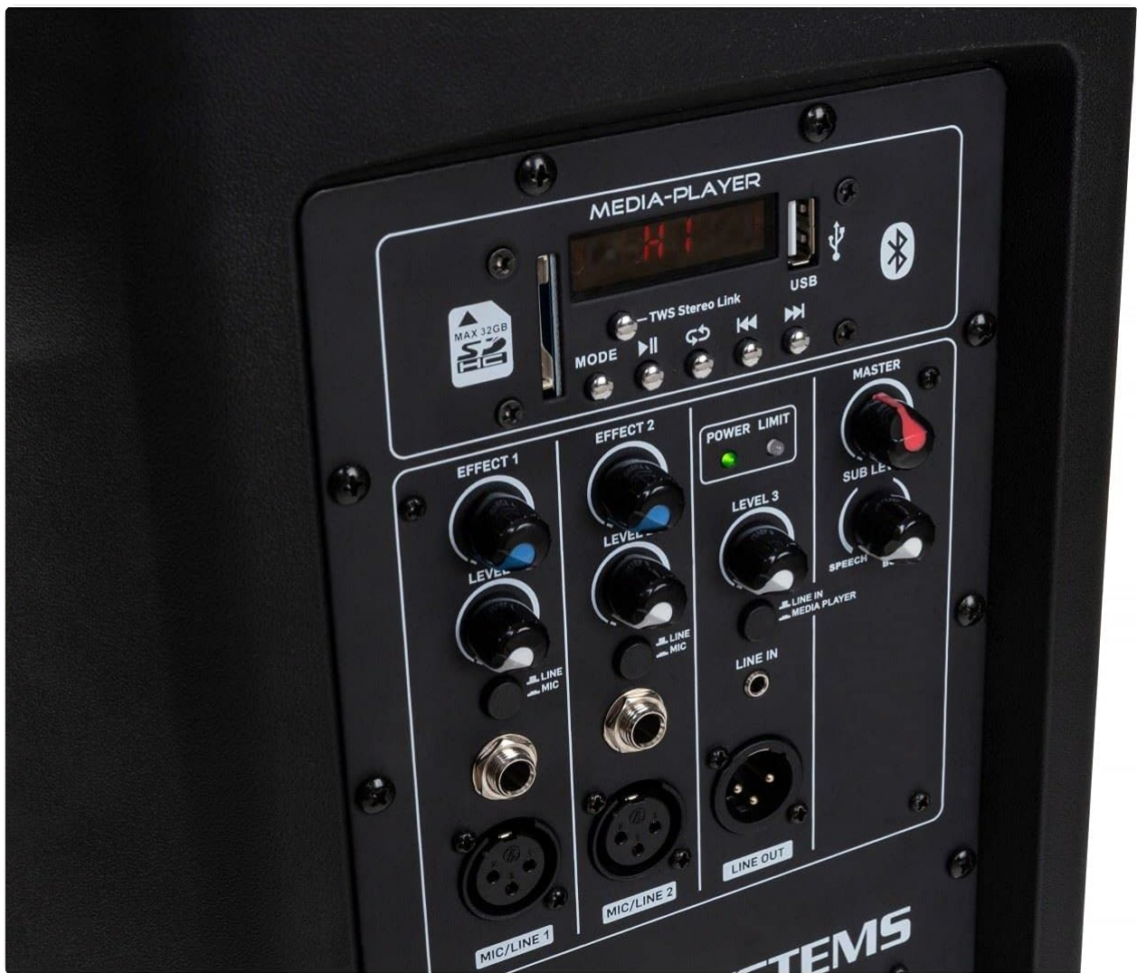
Close-up of the control panel, featuring inputs, level controls, and media player interface.
