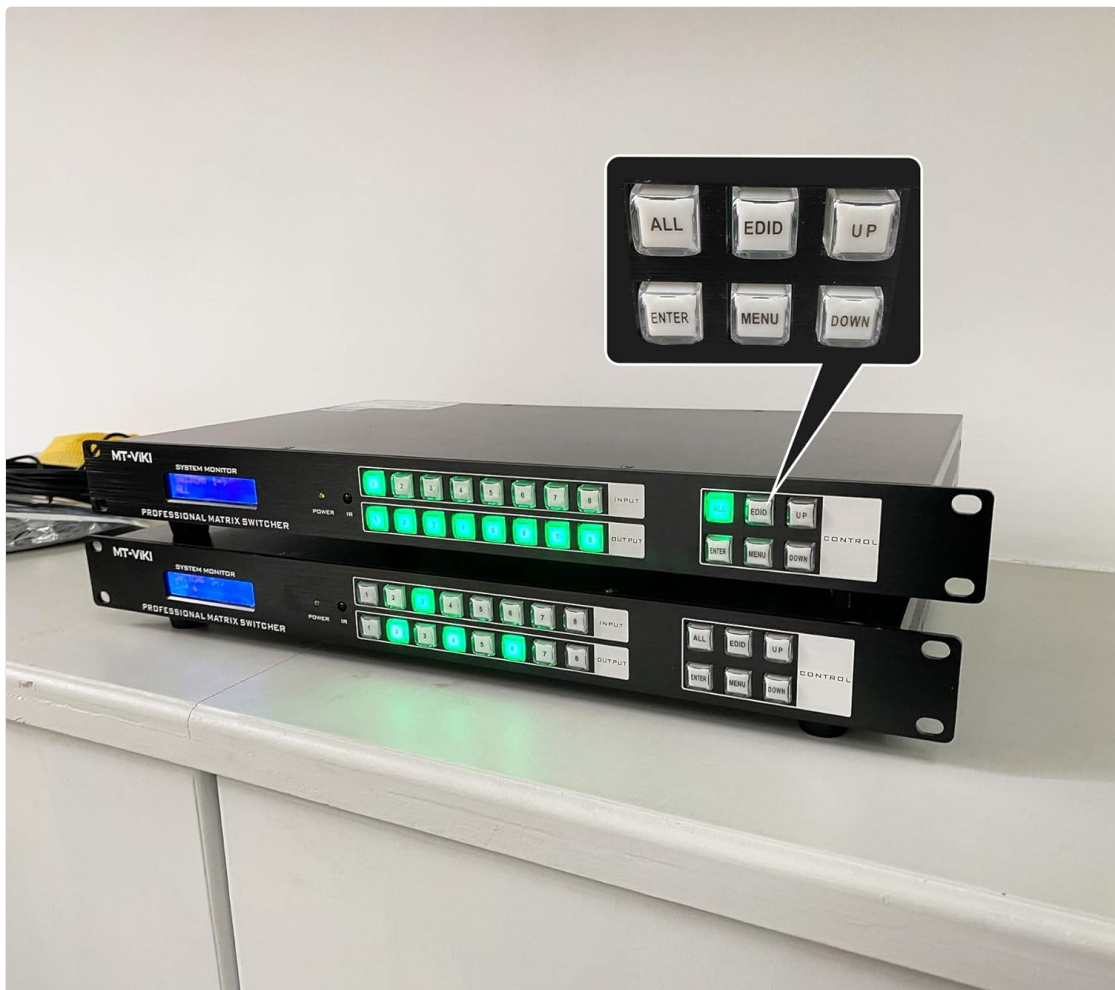
Image 3.1: MT-VIKI HDMI Matrix Switch and its accessories.
