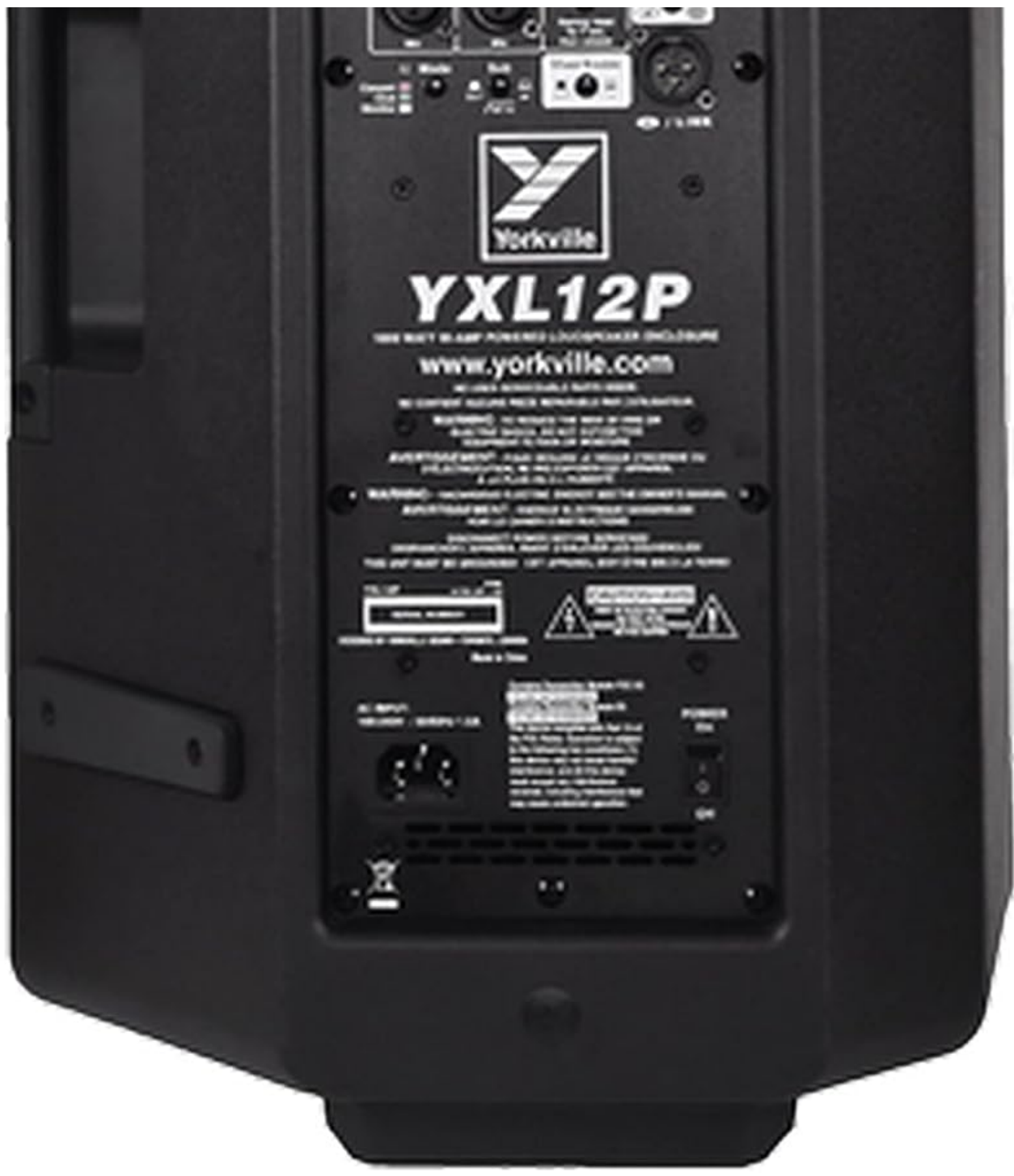
Figure 3.3: Rear panel of the Yorkville YXL12P, showing the various input/output connections and control knobs.
