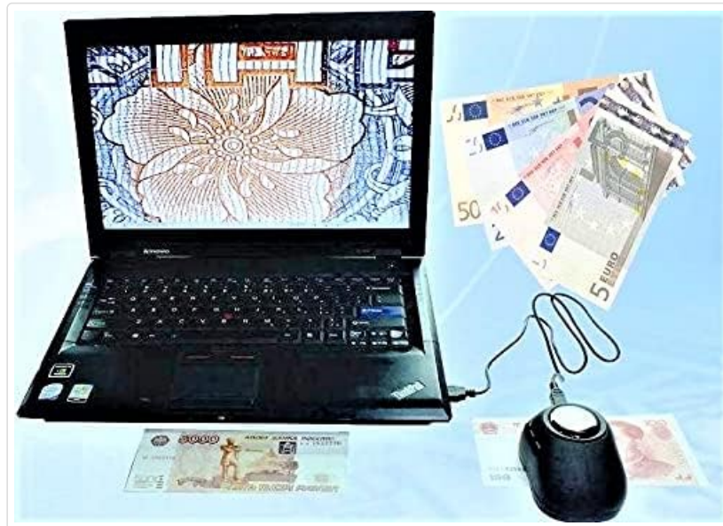
Figure 2.1: Vidia FM-120 connected to a laptop, showing a magnified view of a banknote.
