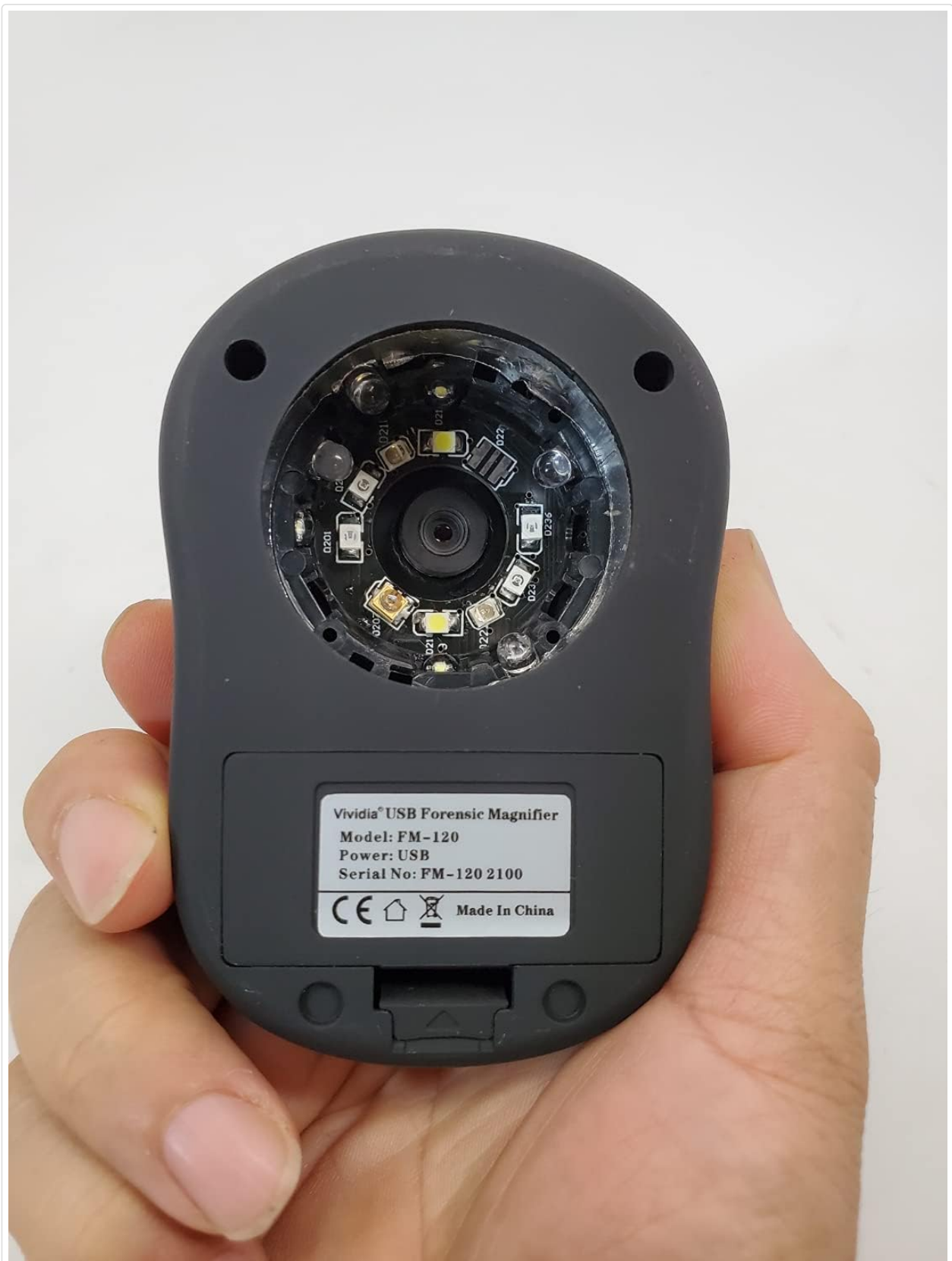
Figure 3.1: Bottom view of the Vividia FM-120, showing the lens and light sources.
