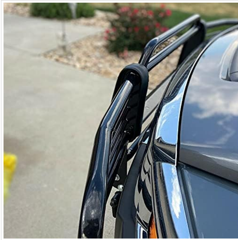
Figure 4.2: Detailed view of the installed grill guard.
