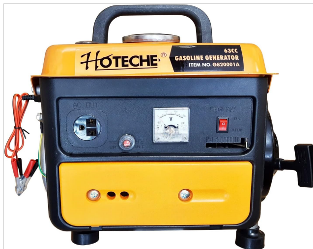
Image 3.1: Front view of the Hoteche G820001A gasoline generator, highlighting the control panel. Key components visible include the AC output socket, voltmeter, engine switch, and choke lever.
