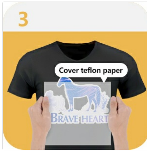
Image: Covering the design with Teflon paper.
